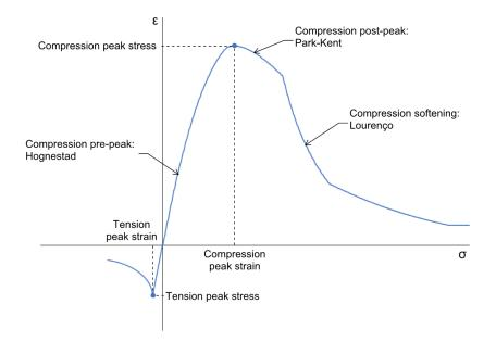
Figure 1. Masonry stress-strain curve
