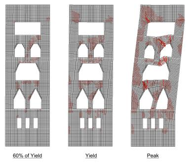
Figure 5. Crack and displacement patterns of a sample wall
