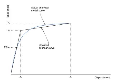
Figure 4. Analytical and idealized force-displacement curves for sample wall
