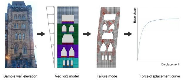
Figure 2. Procedure for determining force-displacement curve for a wall using the VecTor2 software suite
