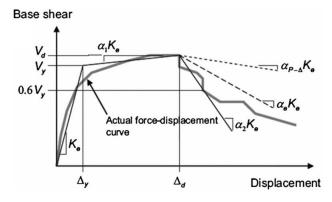
Figure 3. Idealized force-displacement curve [2]
